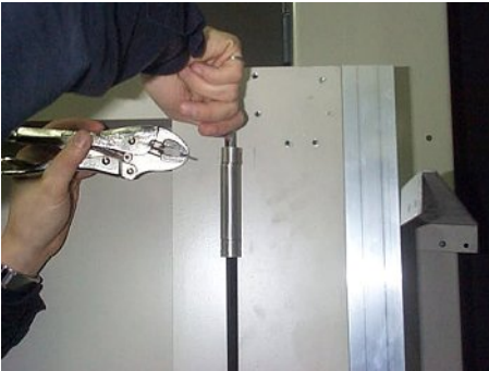
Figure 20 Insert Allen key in hinge and turn to increase tension
