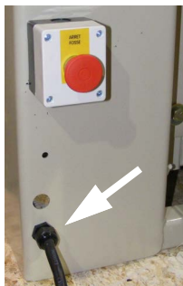
Figure 4 Power cord exiting tower
