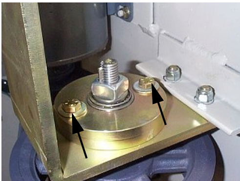
Figure 54 Loosen bolts holding upper bearing disk to L-support
