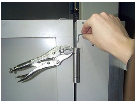
Figure 21 Put pin in place and remove Allen key
