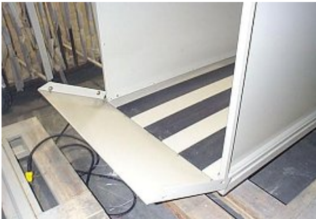
Figure 28 Remove automatic access ramp
