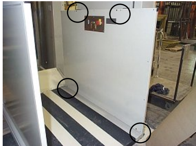
Figure 34 Remove side panel on tower side
