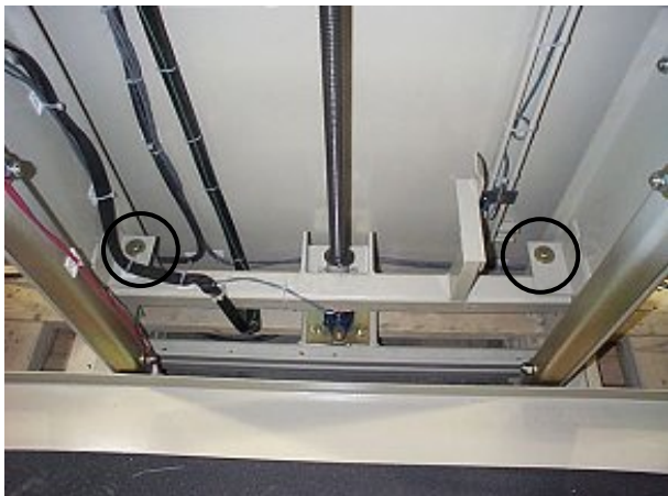
Figure 39 Remove bolts holding roller supports to crossmember
