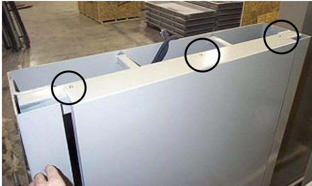
Figure 37 Remove front panel
