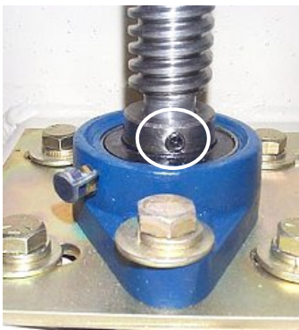
Figure 44 Loosen set screws holding acme screw in lower pillow block
